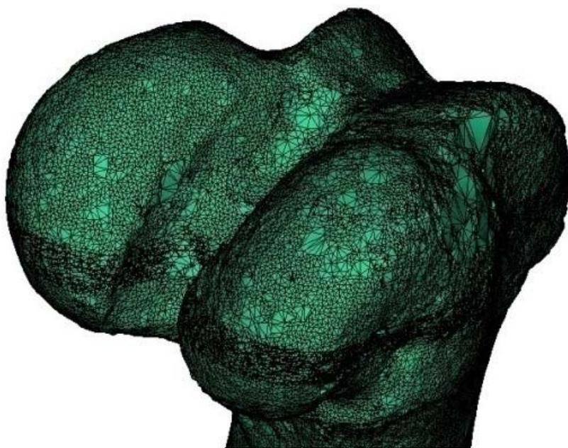
*Finite element model, constructed from laser scanning, of a sheep's knee, for optimisation of articulating surface implant geometry.*
